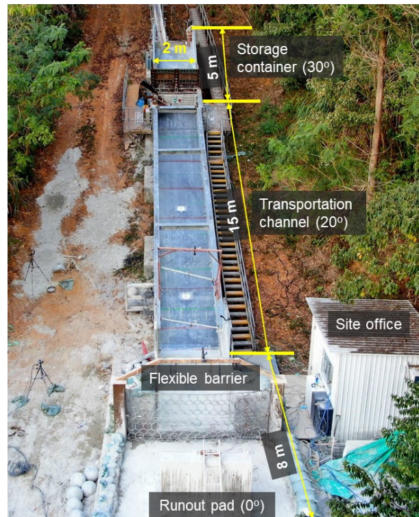
Figure 1. 28-m-long flume at Kadoorie Centre in Hong Kong.
