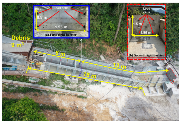
Figure 2. Dual rigid barrier model setup in the 28 m-long flume (inset (a) shows details of the first model rigid barrier; and inset (b) shows the second model rigid barrier).
