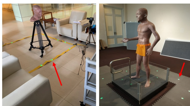
Figure 7. Infrared tracking system (arrowed).
