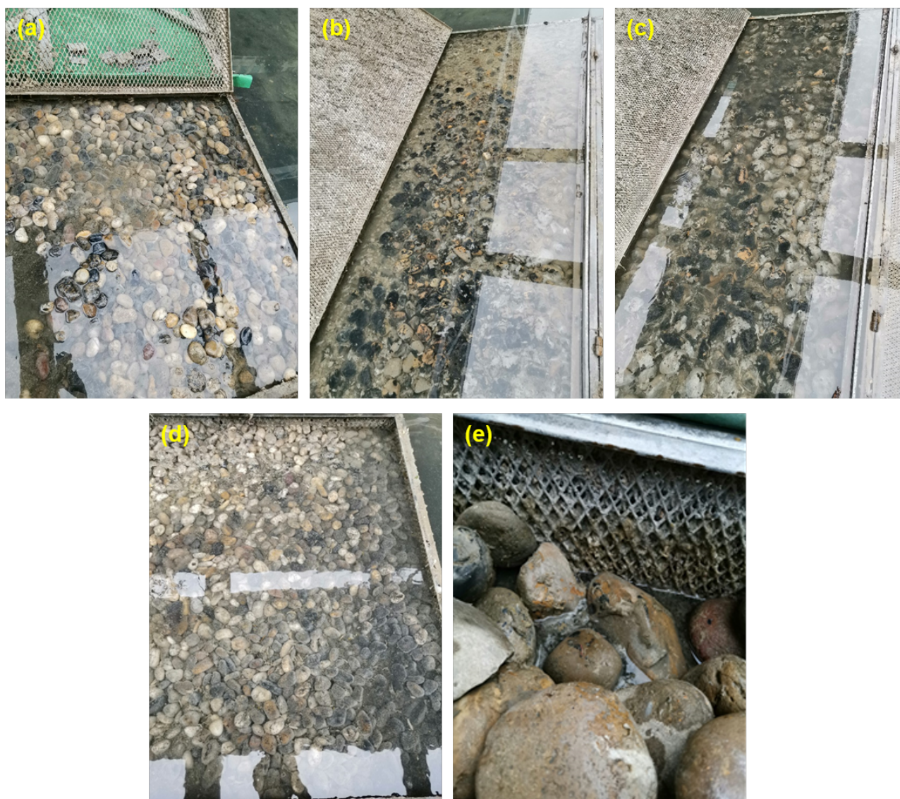
Figure 4. Filter clogging observed in the four filter modules (a-d) and between the cage net (e) after the fourth week of the Round 1 site trial test.
