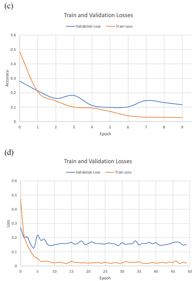
Figure 7. Training and validation accuracies for (a) 10 epochs; and (b) 50 epochs. Training and validation losses for (c) 10 epochs; and (d) 50 epochs.
