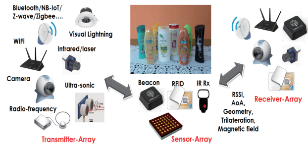
Figure 3. Types of transmitter/sensor/receiver for localisation, positioning and communication of objects.
