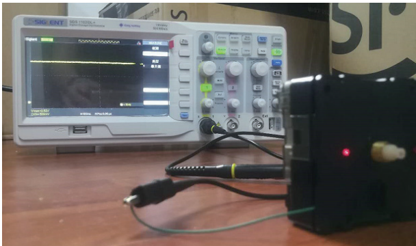
Figure 27. Manchester Coding Signal Transmission using an infrared laser beam.
