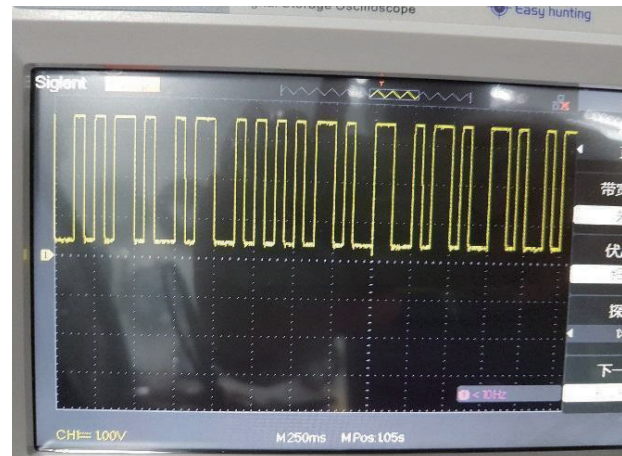
Figure 27. Manchester Coding Signal Transmission using an infrared laser beam.
