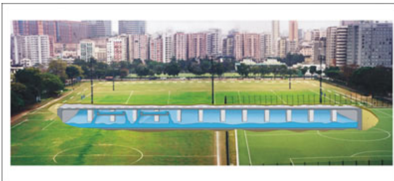
Figure 1 Artist's Impression of the Underground Flood Alleviation Scheme 圖1 地下防洪計劃示意圖
